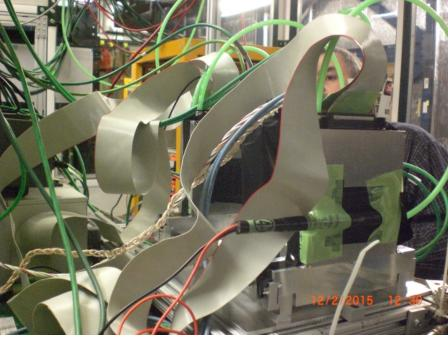
Notice the power supply connections are twisted wire pairs.
