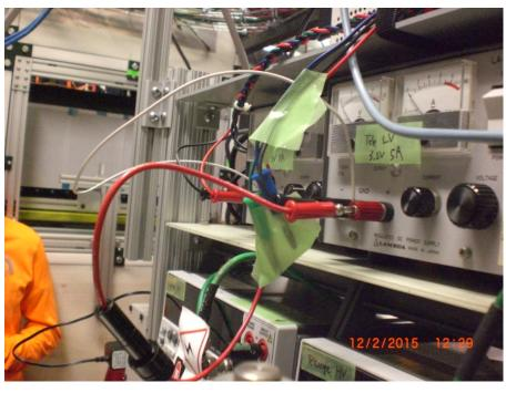
Notice that some power supplies have inline fuses installed at the output terminals.
