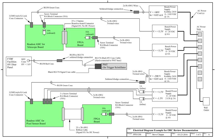
This diagram for the DC and AC power usage can now answer the questions as listed previously. Having this information while visually inspecting an installation allows the ORC review to proceed more efficiently.
